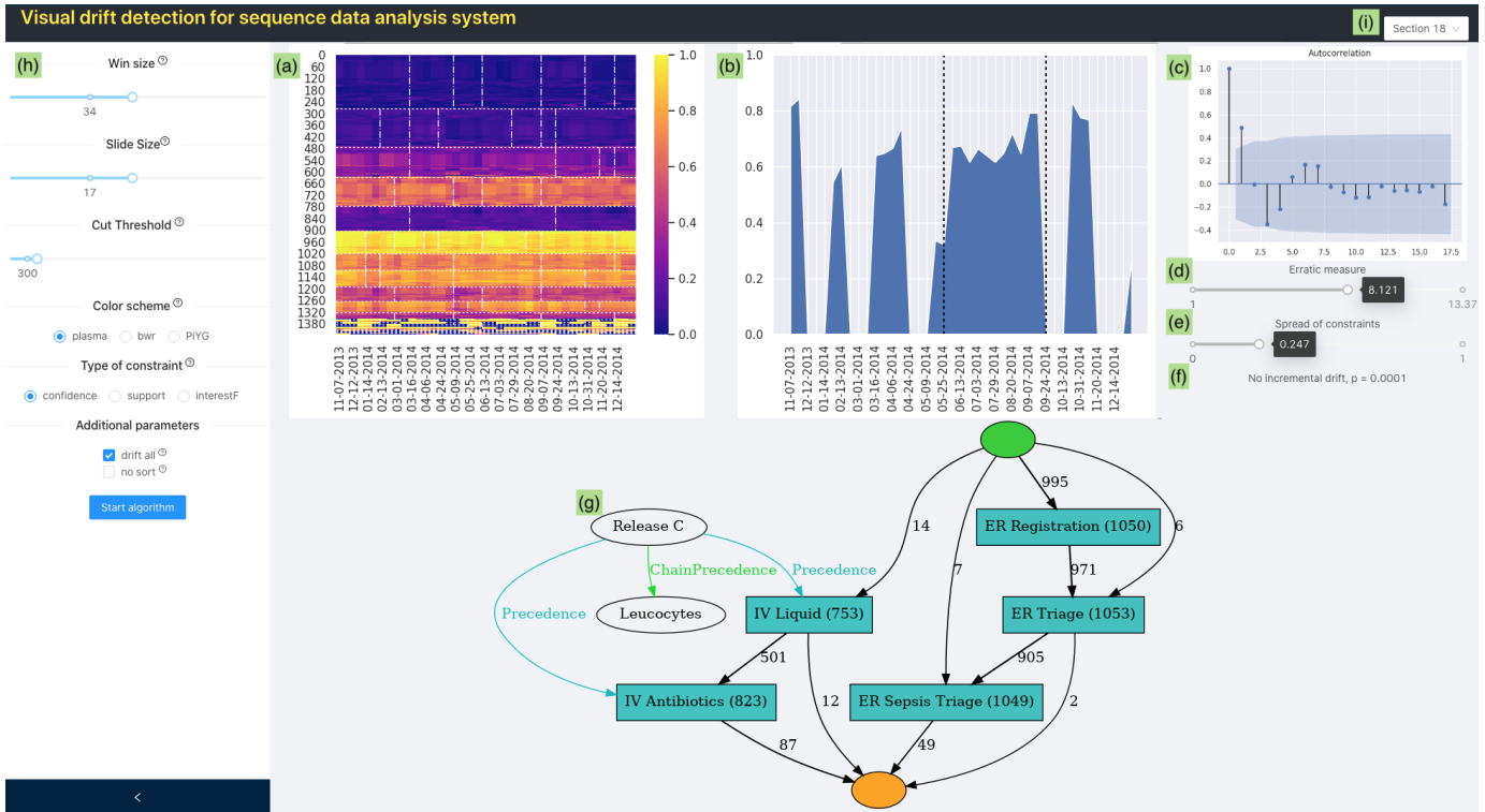
Figure 2: The user interface of the VDD system, running on the Sepsis event log [13]. (a) Drift Map. (b) Drift Chart. (c) Autocorrelation plot. (d) Erratic measure. (e) Spread of constraints view. (f) Incremental drifts test. (g) Extended Directly-Follows Graph. (i) Behavior cluster selection menu.
