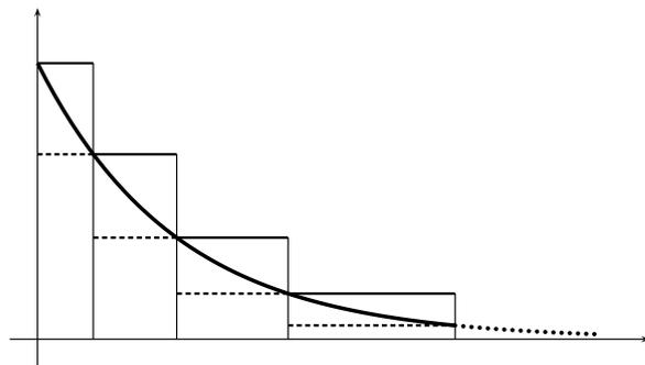
Figure 2. Piecewise constant hat and squeeze (dashed lines) for the exponential distribution. The tail of the distribution has to be cut off (dotted line).
