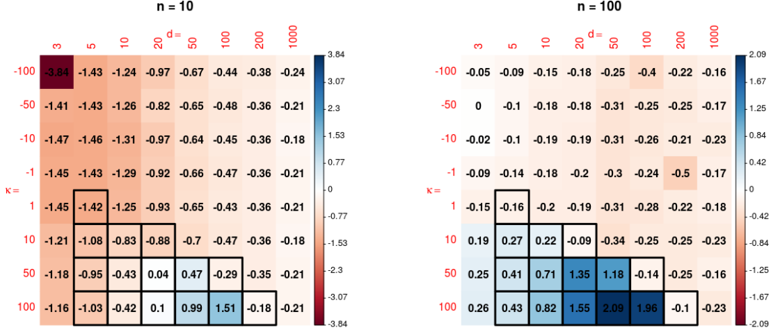
Figure 1: Relative differences of ACG-sampler and Tinflex-sampler for n = 10 and n = 100 , with reference value being the smaller of the two values. Negative and positive numbers (toned into red and blue color respectively) indicate the dominance of ACG-sampler and Tinflex-sampler respectively. Cases where d > 3 and \kappa \geq (d - 3)/2 (i.e., where the log-density of p_{\text{Saw}_d}(g, \lambda) is neither concave nor convex on (0, 1) ) are further annotated with a thick black border.
